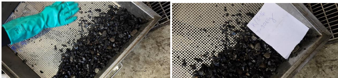
Figure 6 Frost resistance test – preparing samples
